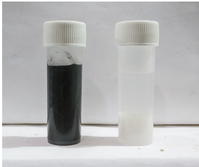
Figure 2.1 Optical pictures of Al NPs in water after mixing (left) and after heating at 95°C for 4 hours.
