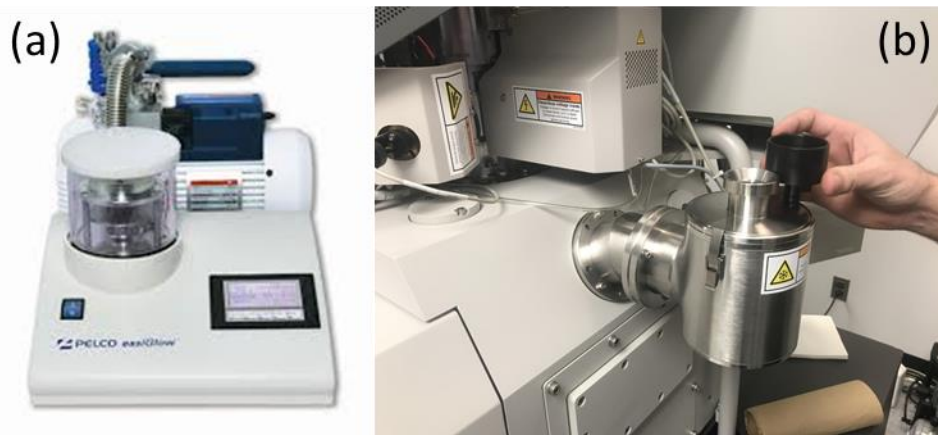
Figure 39. (a) Pelco Easiglow glow discharge cleaning system used for plasma treating SiN E-chips (b) cold trap cooled with liquid nitrogen installed on ESEM to remove contaminants and reduce chamber pressure
