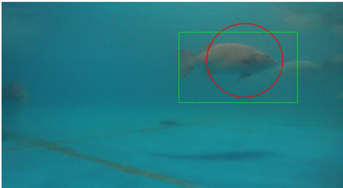
Figure 11. Video 2 with a frame of the fish detection algorithm. correctly detecting a fish in a difficult image. The small differences in the image tones, turbidity, noise and multiple fish in invalid positions present serious challenges that the classifier is able to overcome. The detected fish is highlighted in red, and the candidate ROI in green.
