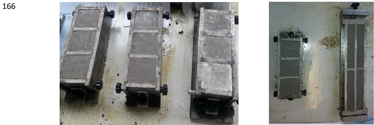
167 Figure 5: Brick samples at the time of casting.
