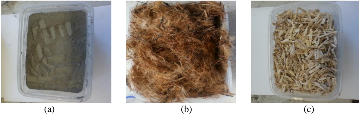
Figure 2: (a) Soil, (b) chicken feather fibres (CFF), (c) sugarcane bagasse fibres (SBF).
