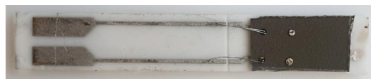
Figure 11. Photograph of the sample chip with ohmic contacts mounted on a ceramics carrier.
