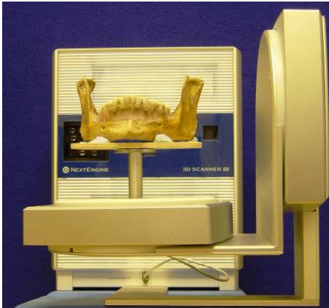
Figure 3.2 Next Engine HD laser scanner and multidrive automated turntable with mandible attached.
