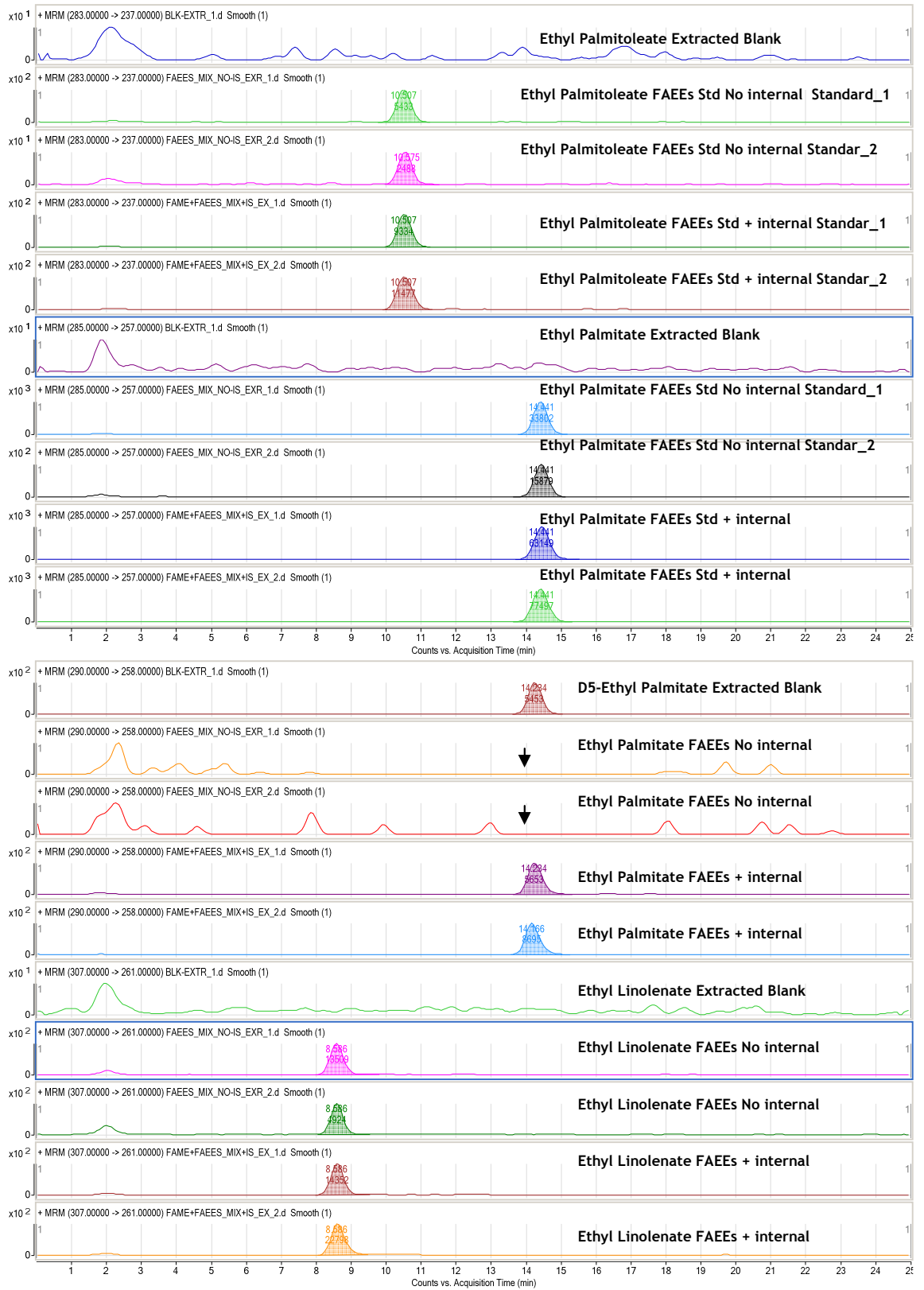
Figure 6-6: Extracted FAEs With and Without Internal Standard. [The arrow indicated no contribution from analyte to internal standard]
