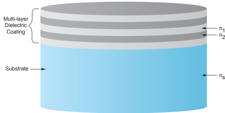
Figure 3.1: Schematic of a multiple layer dielectric stack coating with alternating layers of refractive index n_1 and n_2 respectively, attached to a substrate material with refractive index n_s . Typical coatings have 20 to 32 pairs of layers.
