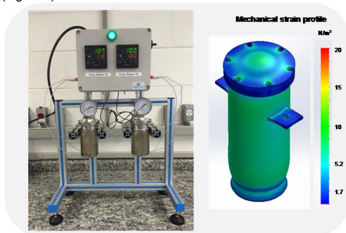
Figure 1: Scheme of the reaction system used in the step3. Mechanical strain and sprain profiles are presented
