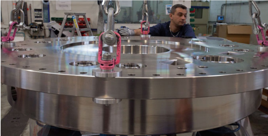
Fig. 26.27 Machined flange of the first Torus Cryo-pump
