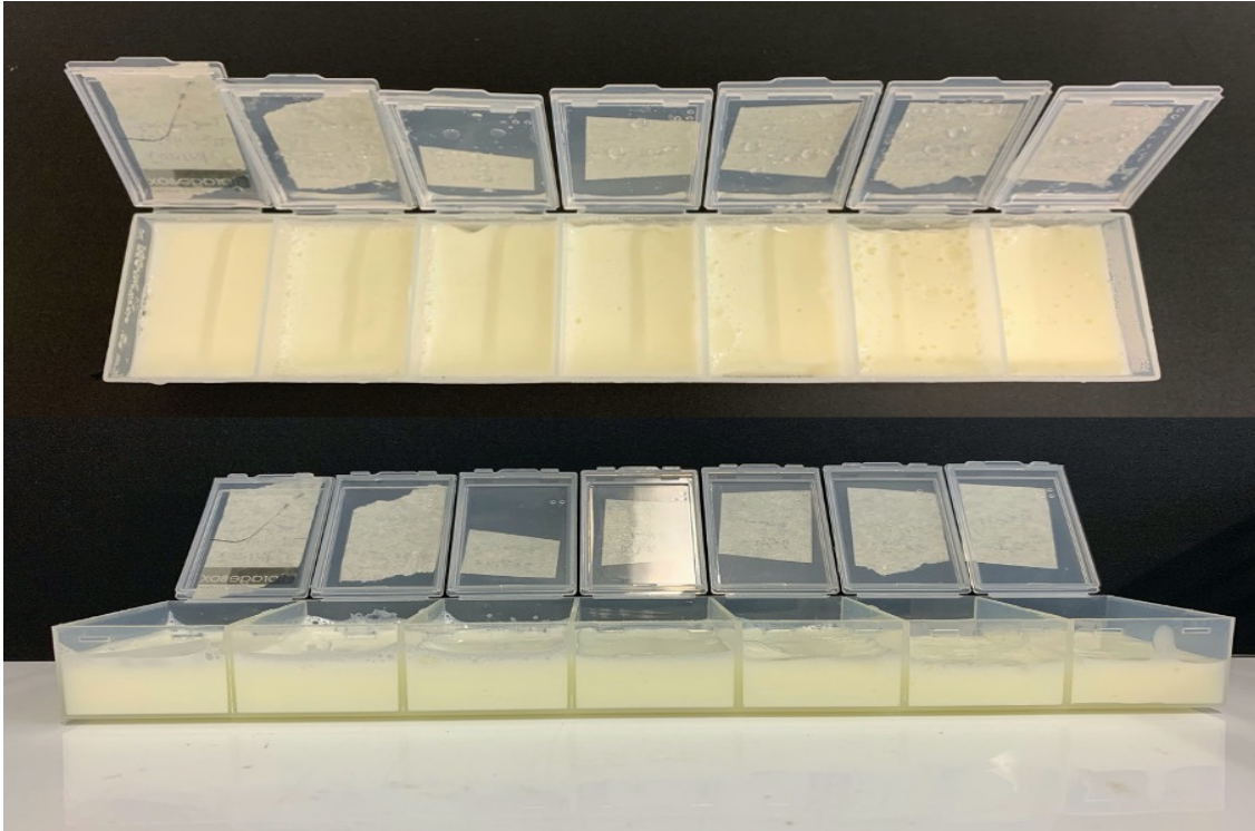
Figure 5.3 The rectangular plastic moulds used for heat treatment and evaluation of any gel formation in skim milk plus calcium lactate samples.
