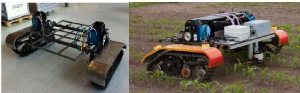
Figure 15: Armadillo track assemble and during operation [15]
