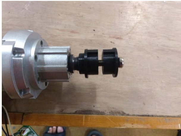
Figure 52: Coupling design attached to the drill
