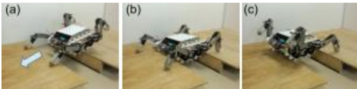
Figure 36: A track leg robot prototype tackling a gap [7]
