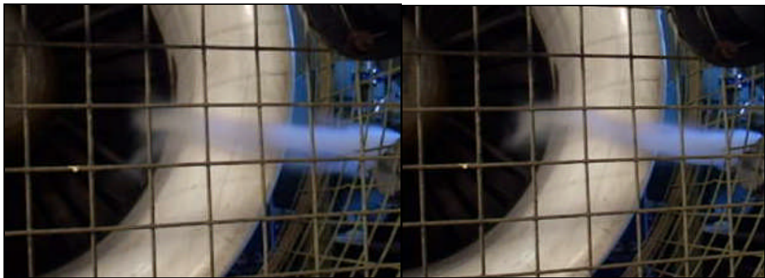
Figure 3–69: Smoke injection at 3 o'clock inlet position.
