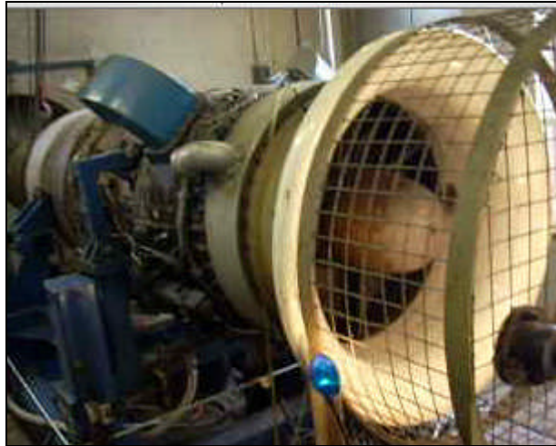
Figure 3–66: Rolls-Royce Avon jet engine.
