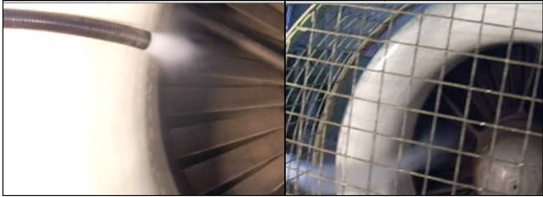
Figure 3–68: Smoke injection at 9 o'clock inlet position.
