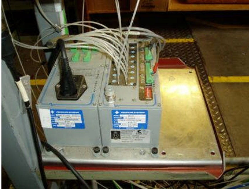
Figure 4–38: Chell 9000 Intelligent Pressure scanners rated at 30 psi.
