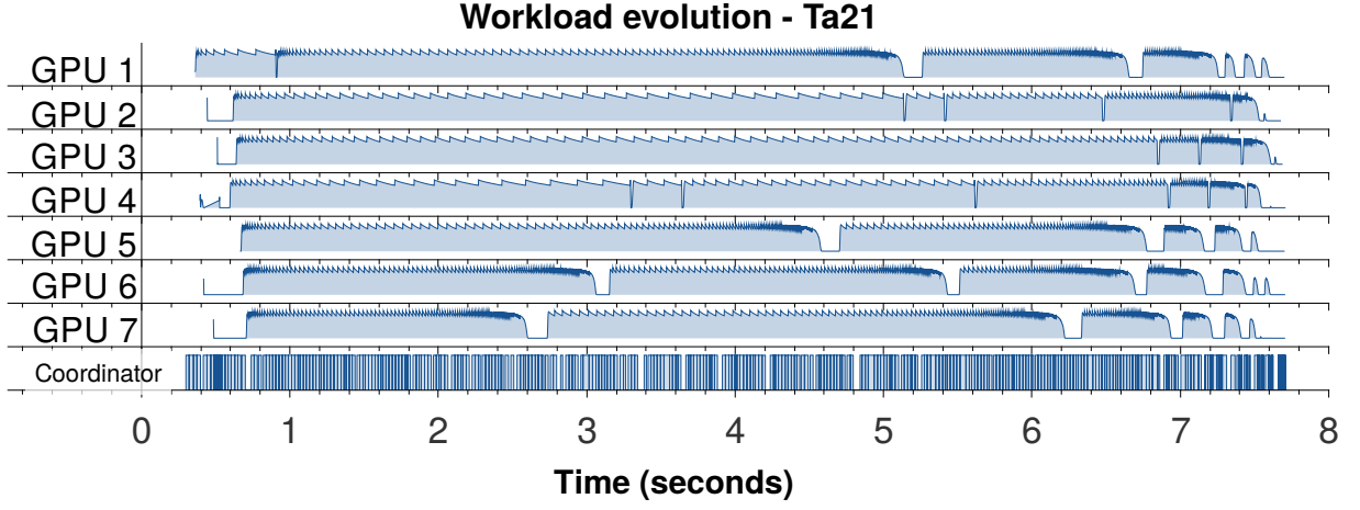
Figure 10: Evolution of workload during resolution of instance Ta021 (461M explored nodes) on 7 GPUs. The horizontal axis represents the elapsed time (in seconds).
