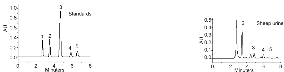
Figure 1 Chromatograms of PD and creatinine in standards and sheep urine. 1. allantoin; 2. creatinine; 3. uric acid; 4. hypoxanthine; 5. xanthine
