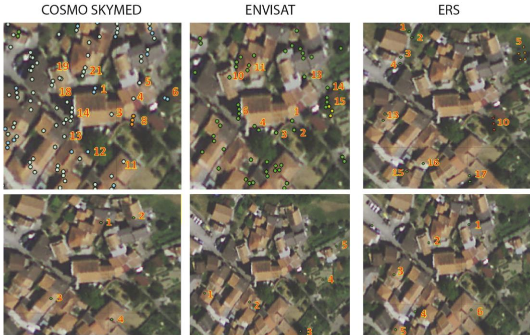
Figure 21 – Target available for all the SAR satellite (CH_32), respectively on the top ascending and on the bottom descending orbits
