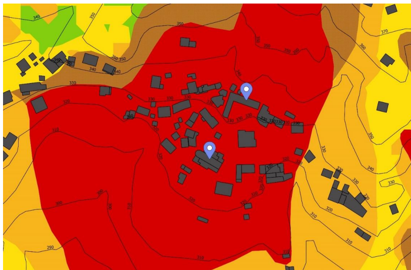
Figure 17 - Identification of churches located on active landslide areas: the case of Sant'Olcese church (GE).
