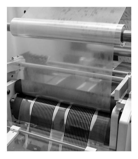
Figure 4.8: Illustration of hot lamination process. Reproduced from [70] with permission from Elsevier.
