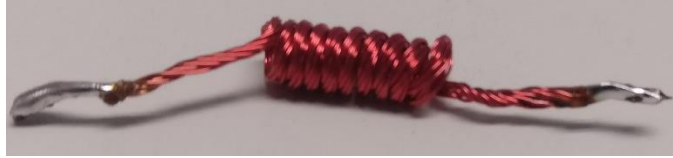
Figure 3.12. 50 nH air-core inductor.
