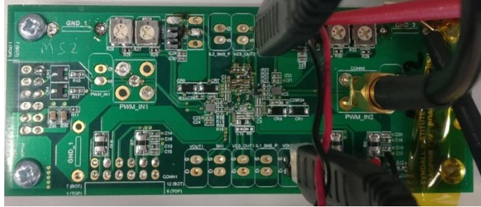
Figure 4.2. Circuit board set-up for later “full-converter” measurements. Inductor device mounted on underside of PCB, EPC3 MS2 circuit board.
