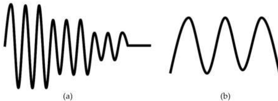
Figure 3: (a) Bending instability from previous studies and (b) expected surface topography of the sample
