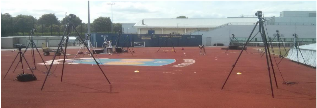
Figure 3.2 Motion capture system (Qualisys) set up configuration with 12 motion analysis cameras and one video camera. Calibrated to 2.6mm error over a capture area of 15x3m
