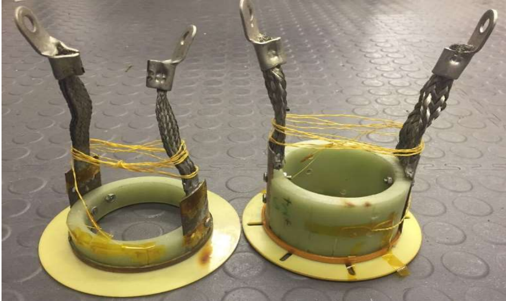
Figure 6.1 Multi-filament sample coil (left) and non-striated sample coil (right) wound by YBCO coated conductors supplied by the SuperPower.
