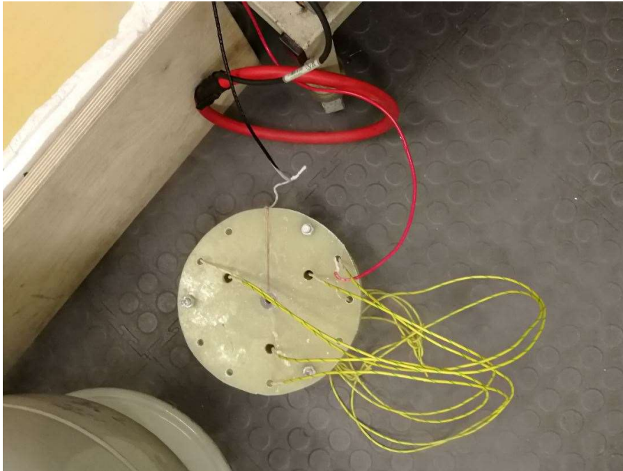
Figure 5.4: Magnetisation copper coils held by G10. Plastic wires are bonded through the holes drilled in the G10 holders for lifting and moving the magnetisation system in and out of the liquid nitrogen tank conveniently.
