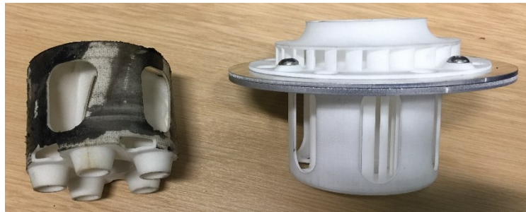
Figure 8-11 M/G unit internal cooling fan. The fan on the left is the old design while the fan on the right is the improved design, courtesy Ashwoods Motors
