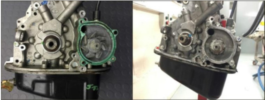
Figure 6-9 Mechanical coolant pump before and after removal of impeller blades [2]
