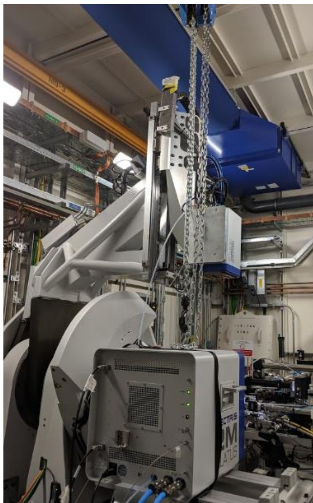
Figure 5.14 – Dectris 2M PILATUS detector employed for beamtime experiments (PCMKS).
