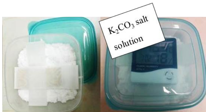
Figure 6.6 – Inside of humidity ageing unit containing raised ledge for humidity sensor (left) and humidity sensor within sealed plastic container containing salt solution slurry (right).
