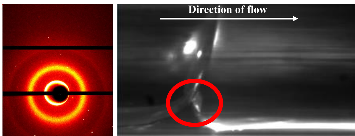
Figure 5.24 – 2D diffraction frame showing diffraction spots (left) with the corresponding solution slug held in the X-ray beam during data collection, captured by a camera positioned by the X-ray beam (right), the single crystal is positioned at the back of the solution slug highlighted by the red circle.
