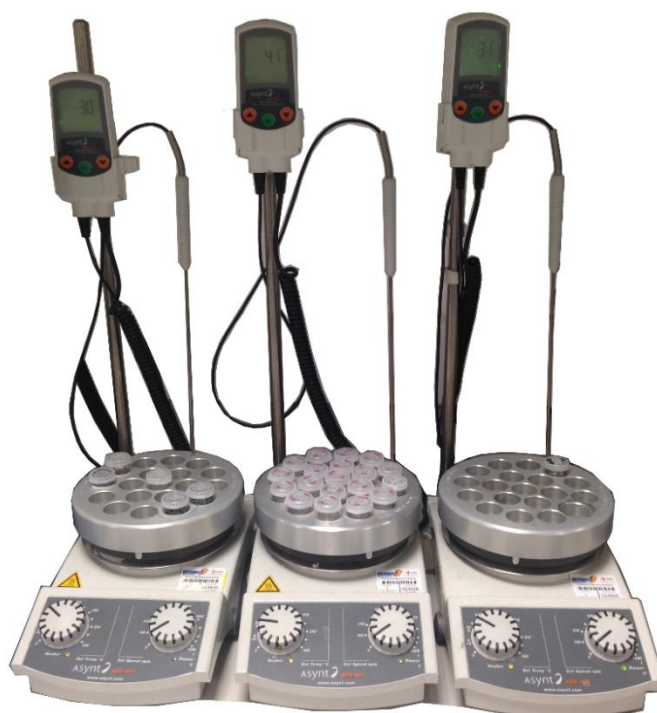
Figure 6.4 – Welled DrySyn forms fitted on hot-plates for crystallisation via evaporation of the solvent at elevated temperatures of 30, 40 and 50 °C.
