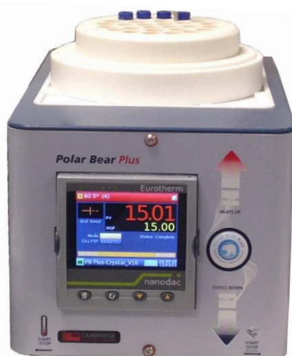
Figure 6.5 – Cambridge Reactor Design (CRD) Polar Bear Plus crystalliser for temperature controlled batch cooling crystallisations.
