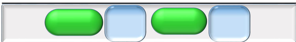
Figure 1.23 – Segmented flow comprising three immiscible media: media 1 (green), media 2 (blue) and media 3 fills the inside of the tubing (off-white).
