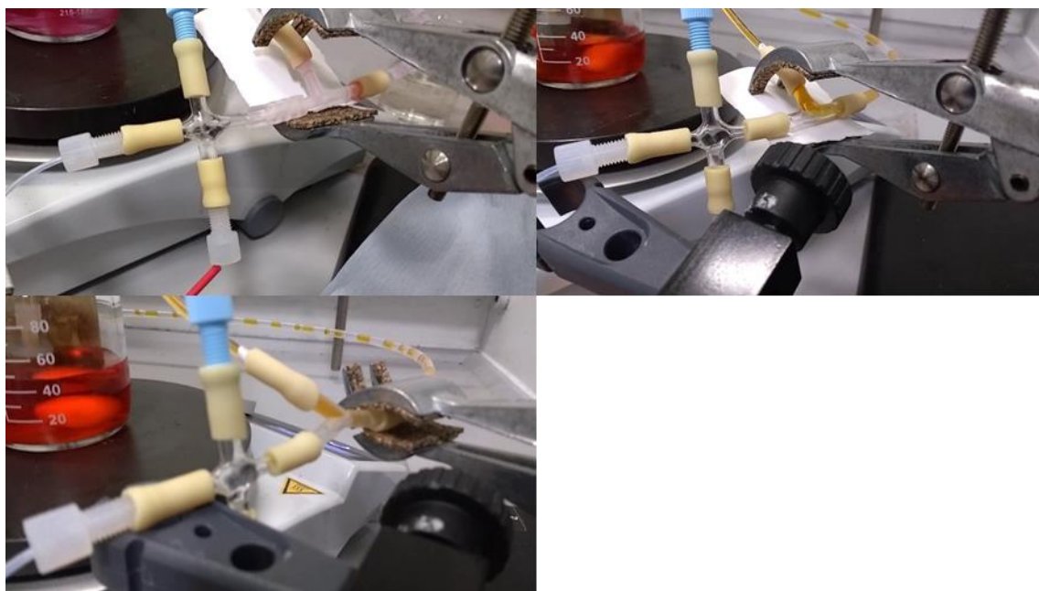
Figure 4.7 – Images of segmentation X-piece connected to (clockwise) PP T-piece, glass T-piece and PP Y-piece seed / dye inlet connectors for seeding optimisation studies.
