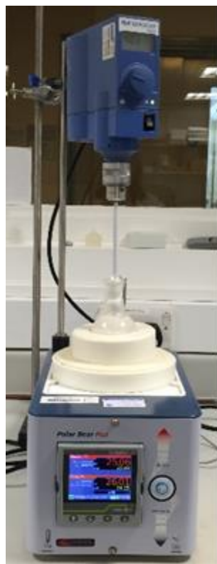
Figure 3.3 – The Cambridge Reactor Designs (CRD) Polar Bear Plus Crystalliser, featuring overhead stirring.
