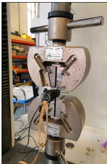
Figure 4.26 Experimental Instron 3369 load cell set up with clip-gauge extensometer attached.
