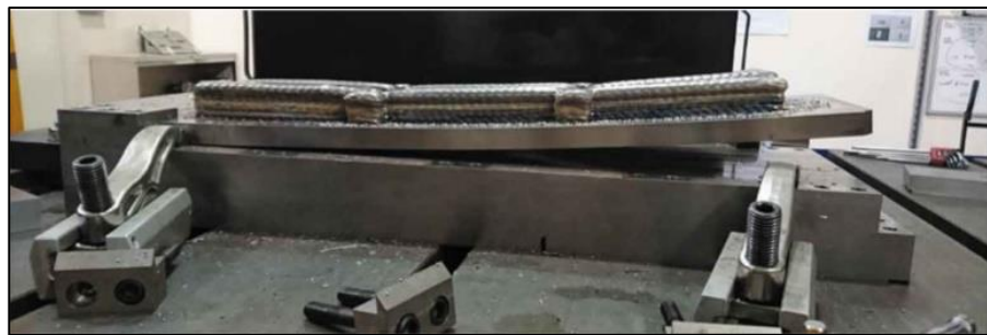
Figure 1.4 Structural distortion of a WAAM part due to residual stress (Xu et al., 2018a)
