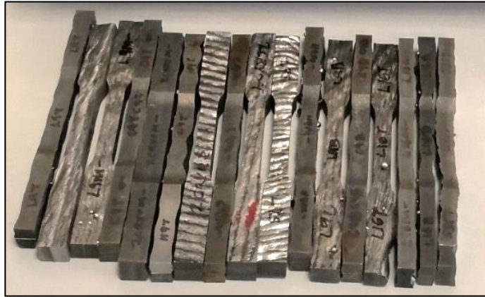
Figure 4.23 Pre-machined condition of the tensile samples for density measurement.
