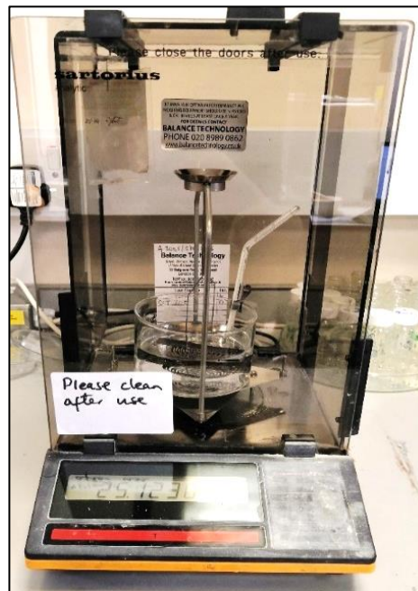
Figure 4.24 A120S Analytical Balance Scale with Sartorius™ Balance Density Determination Kit b) Pre-machined test condition of the tensile samples before CNC machining.
