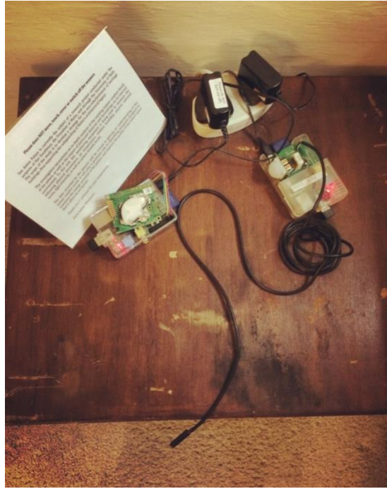
Figure 5.14: Data loggers monitoring environmental parameters at San Anton Palace (Source: A Wismayer)
