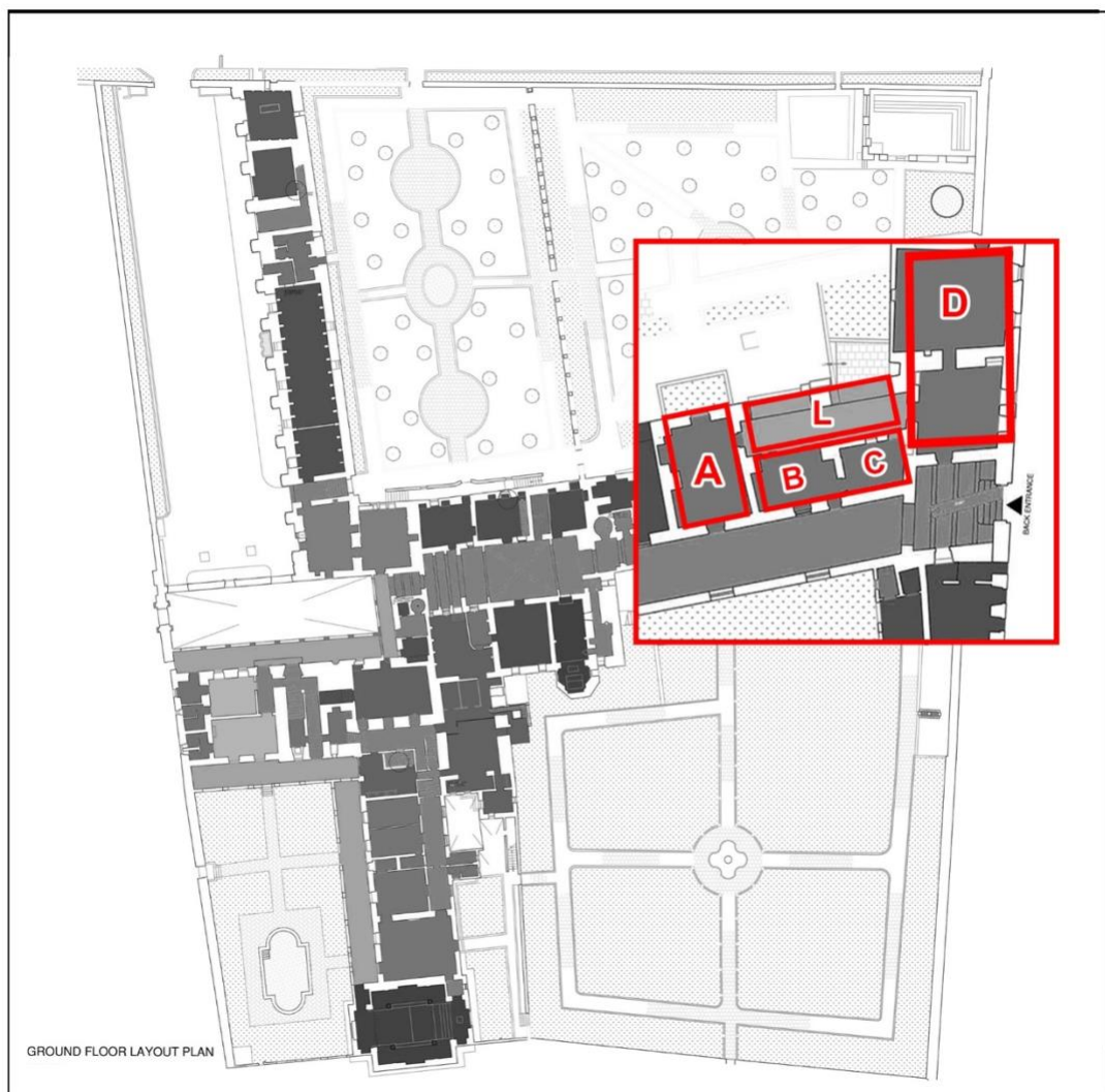
Figure 4.3: Data loggers were installed in offices (rooms A-D) at ground floor level
