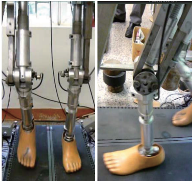
Figure 2.29: Two leg lower prostheses walker and its force test table [88]
