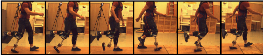
Figure 2.22: An example of testing with modified prosthetic knee simulator [69]
