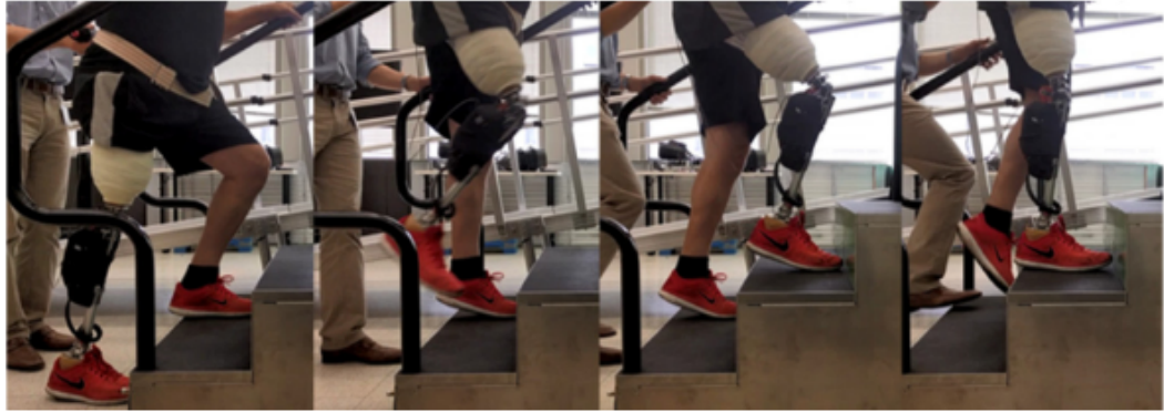
Figure 2.20: An example of amputee testing transfemoral prosthesis [13]
