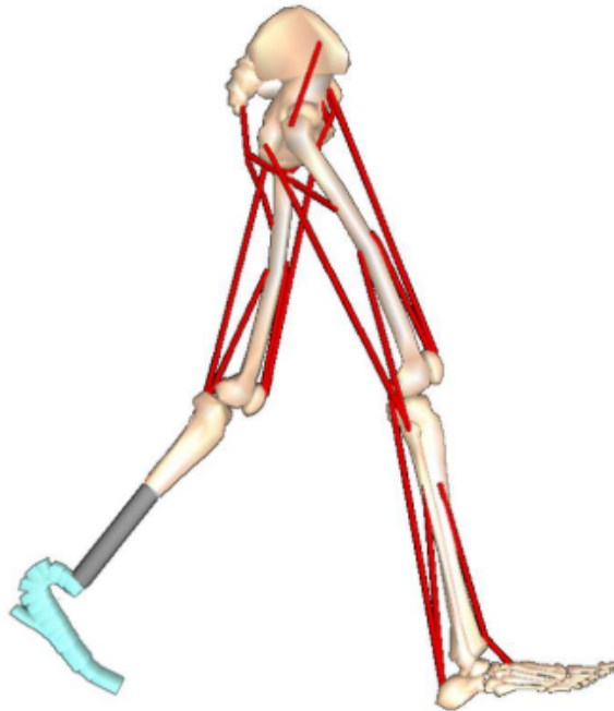
Figure 2.19: Lower-limb amputee musculoskeletal model with a prostehsis [12].
