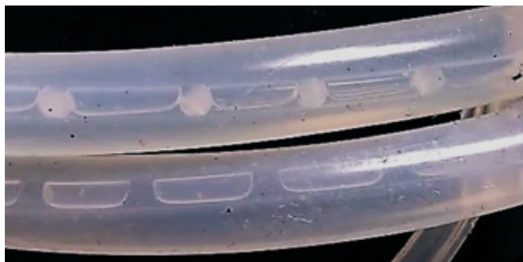
Figure 4-11: Initial nucleation within the cooled J2 tubing jacket during controlled nucleation run, PZA7. Crystal growth becomes visible to the naked eye within the upper rung of the cooling jacket.
