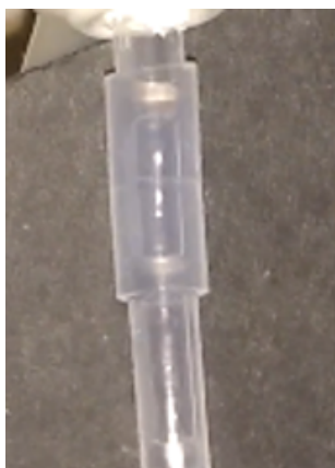
Figure 4-19: Union between Jacket 2 (J2) and the 15 m FEP tubing in the KRAIC
