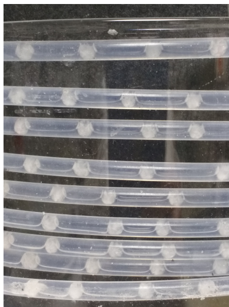
Figure 4-21: Crystallisation of pyrazinamide in all slugs in coil 1 of the KRAIC in PZA10
