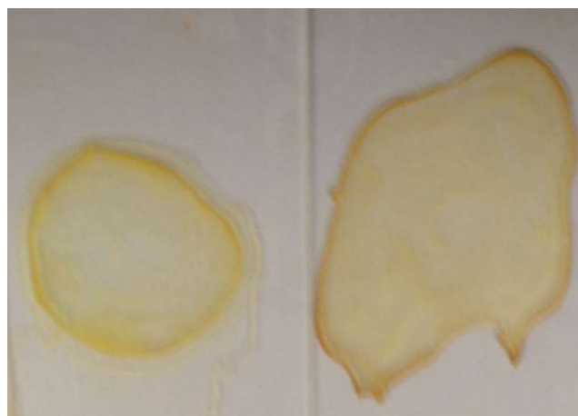
Figure 7.26: LHS: Thin film of Complex 30 , deposited from a concentrated MeOH solution. RHS: Thin film of complex 30 after exposure to acidic vapour.
