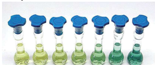
Figure 1.25: Change in colour on the addition of diethyl ether to a terpyridine complex. 61
