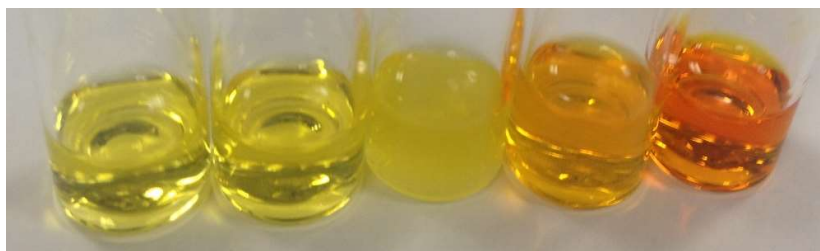
Figure 7.23: pH-sensing capabilities of complex 30 , all solution in methanol. From right to left: Vial 1 with 2 drops of tolyl-sulphonic acid, Vial 2 with two drops of HCl, Vial 3 with 2 drops of trifluoroacetic acid, Vial 4 Neutral complex, Vial 5 with 2 drops of tri ethyl amine.
