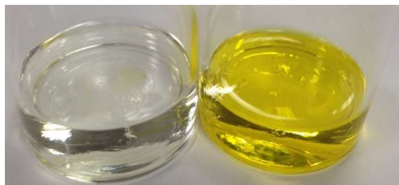
Figure 7.17: Photograph of a solution of Compound 29 before (clear) and after (yellow) acid addition.
