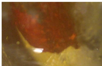
Figure 5.33: Two different solvates of complex 19 , Yellow is the DCM solvate and orange is upon exposure to acetonitrile.
