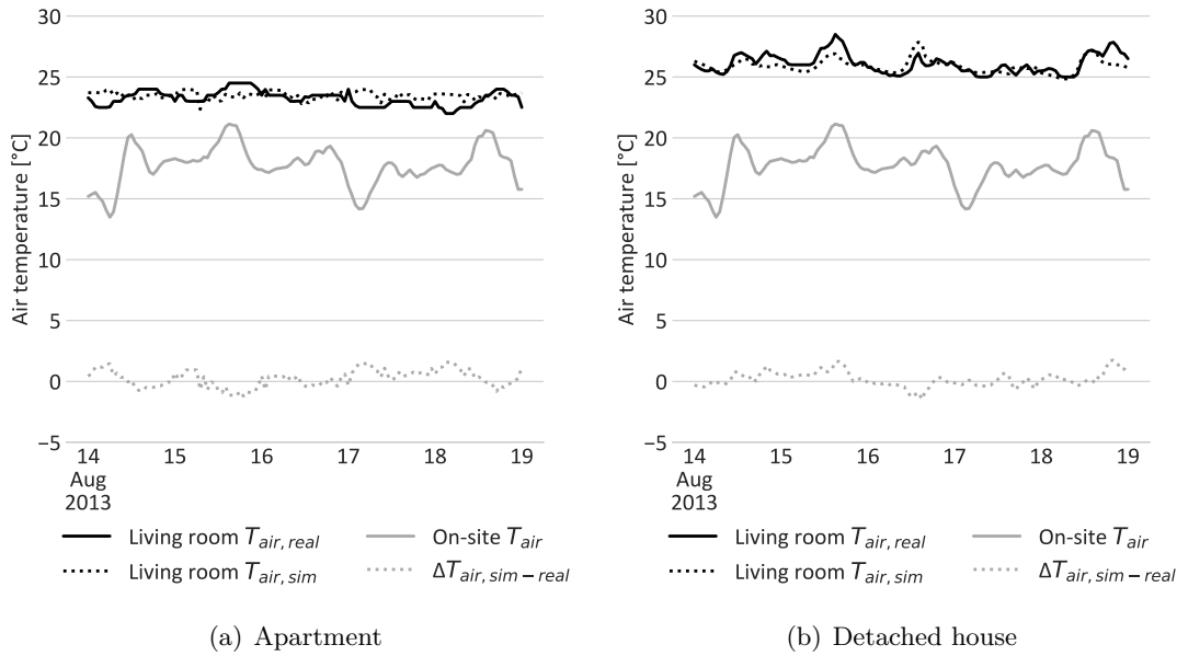
Figure 2.5: Comparison of monitored (real) and base models simulated (sim) internal air temperature (with the model performance assessed via the MBE and the CV(RMSE); see section 2.5.3 for a description of these metrics)
