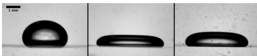
Fig. S7 Images of 24 h aged water droplets containing 0, 55 and 250 mM NaCl, from left to right respectively, in OA-doped oil.
