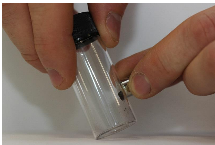
Figure 2.20: Photograph of P5py responding to a bar magnet.
