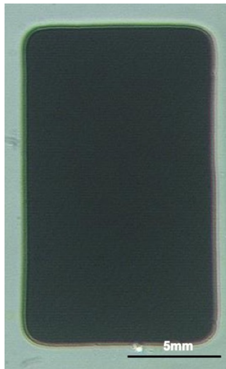
Figure 47. Aluminium-Zinc layer under optical microscope, an n-Plan lens was used.
