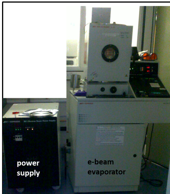
Figure 13. The electron beam evaporator on the right-hand side and its power supply on the left hand side.
