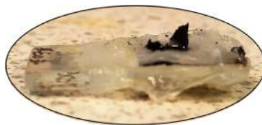
Supplementary Figure 14: Fracture of GS causing water infiltration. Photograph of the device tested at an applied potential of 1.23 V versus RHE. 0.1 M \text{KNO}_3 electrolyte solution pH 7, under continuous simulated solar light irradiation after 23 h of operation under continuous illumination.
