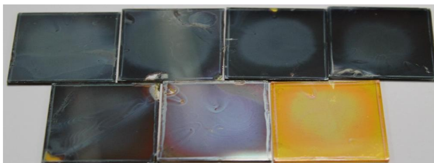
Figure 5.4.1. Photograph of films produced from solutions of varying azetidinium iodide mole percentage, from left to right how they will be referenced from this point on is shown in bold : (top row) MAPI (A0, 0 mol% AzI), 1 mol% AzI ( A1 ), 2 mol % AzI ( A2 ), 5 mol% AzI ( A5 ); (bottom row) 10 mol% AzI ( A10 ), 25 mol% AzI ( A25 ) and AzPI ( A100 , 100 mol% AzI)
