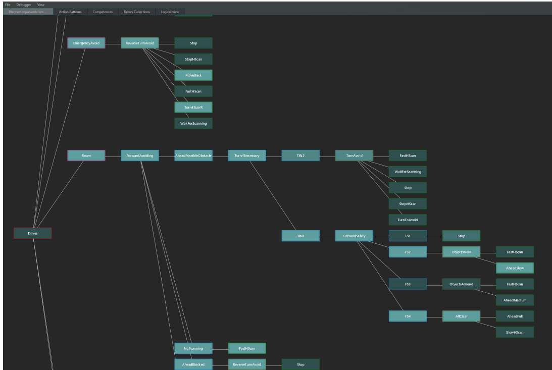
Figure 4-6: The ABOD3 Graphical Transparency Tool displaying an Instinct plan in debugging mode. The highlighted elements are the ones recently called by the planner. The intensity of the glow indicates the number of calls coherent with their recency.
