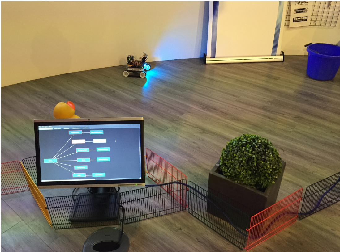
Figure 5-5: Directly Observed Robot Experiment: Photograph showing the R5 robot in a purposed-made den. Obstacles visible include a yellow rubber duck and a blue bucket. The position and orientation of the display is shown, with the ABOD3 opened and visualising the real-time transparency feed from the robot. The display was turned off to create our control group, Group 1 (Wortham, Theodorou and Bryson, 2017a; Wortham, 2018).
