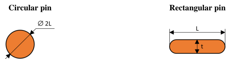
Figure 6.2. Considered pin shapes. The circular section is commonly used whilst a rectangular section is proposed to enhance pin external surface.
