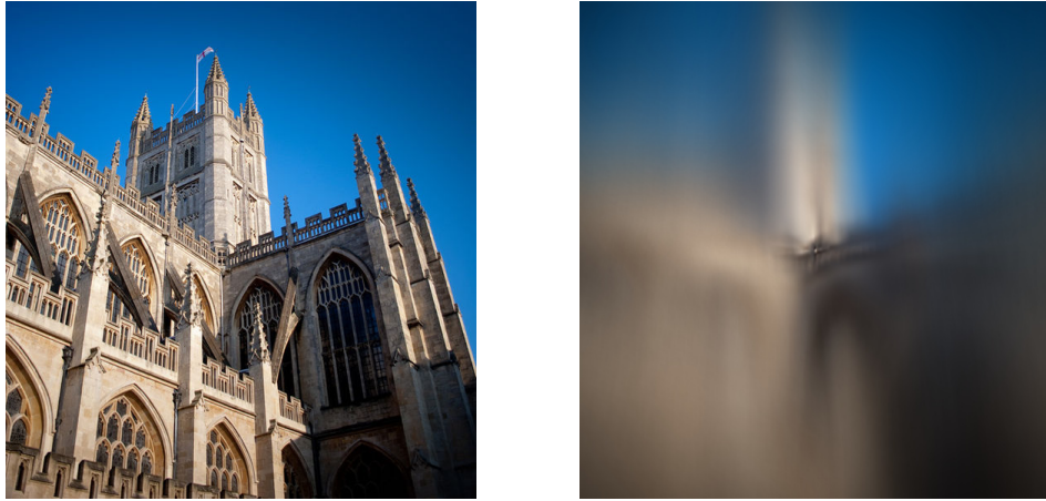
Figure 3.6: Left: original image of Bath Abbey; right: the image produced by averaging the colour values at each pixel location when the original image has been warped by a number of affine transformations centred on the image centre. This results in locations further from the centre of the image being more blurred.
