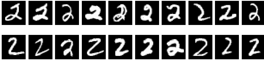
Figure 1.39: Images with the digit two from the the MNIST database: the CNN classifier was able to correctly classify images in the top row but not the bottom row
