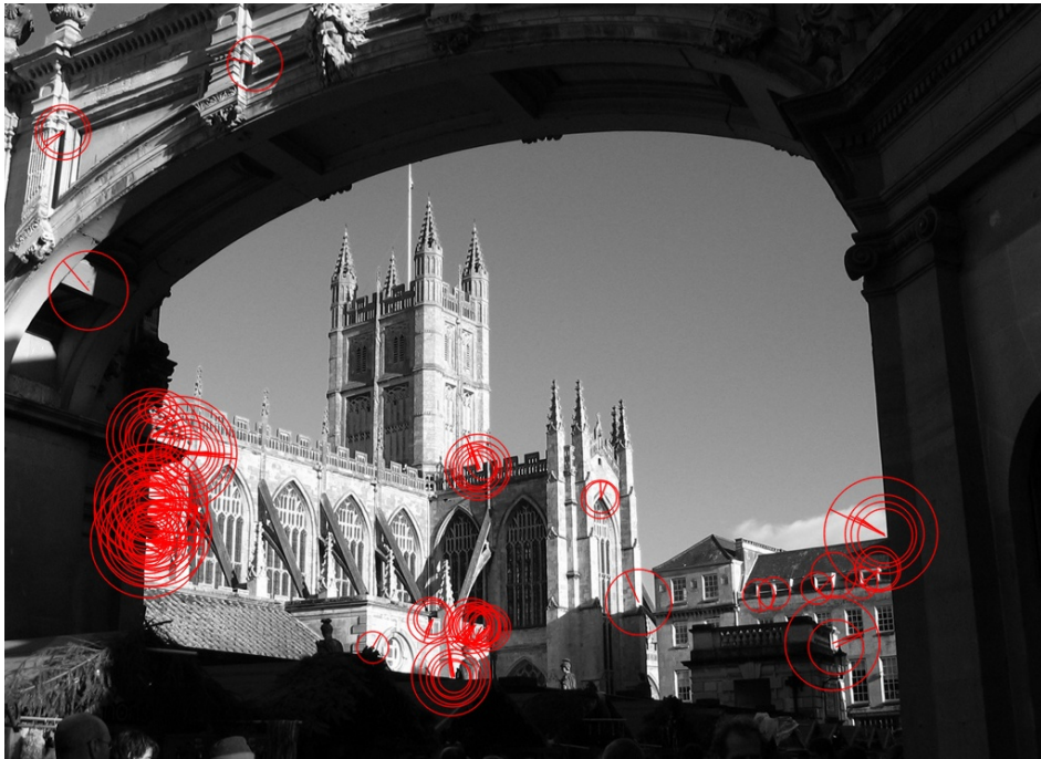
Figure 1.7: ORB interest-points extracted from an image of Bath Abbey: the interest-points are drawn so as to show their relative size and orientation.
