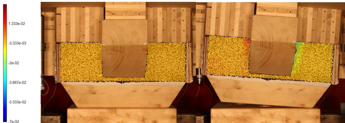
Figure 111 The DIC result for the base Dou connected by a wood peg connection
