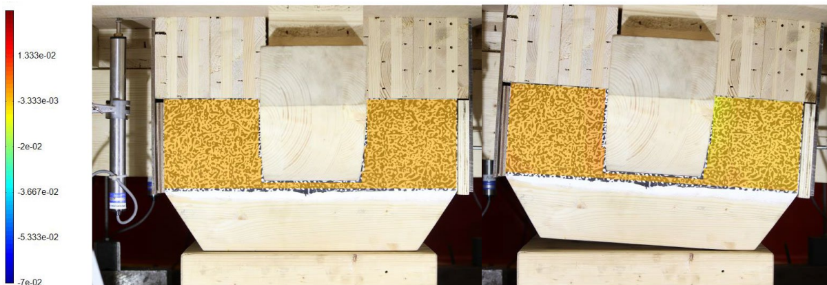
Figure 113 The DIC result for the base Dou connected by a SMA bar connection with 1% prestrain
