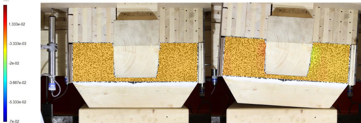
Figure 114 The DIC result for the base Dou connected by a SMA bar connection with 3% prestrain
