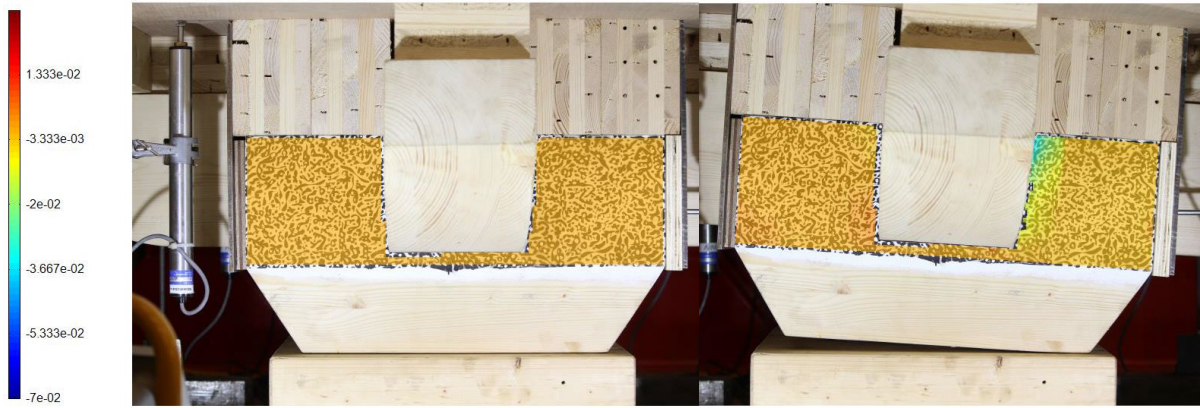
Figure 112 The DIC result for the base Dou connected by a steel bar connection
