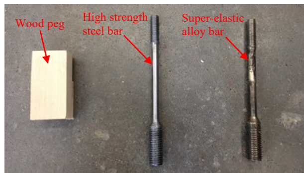
Figure 67: The materials of three different connections
