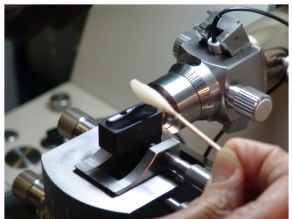
Fig. 7.9 Cotton dipped in alcohol to produce fume to stretch sample
