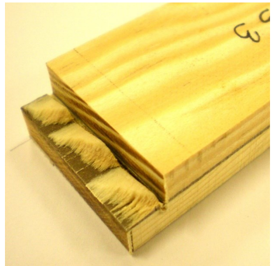
Fig. 10.12. Wood failure of TAST tested Timberset samples with portion of earlywood.
