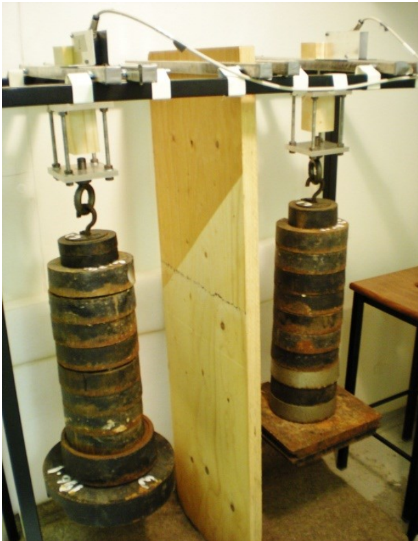
Fig. 12.10 The complete configuration of the creep test in a walk-in humidity chamber
