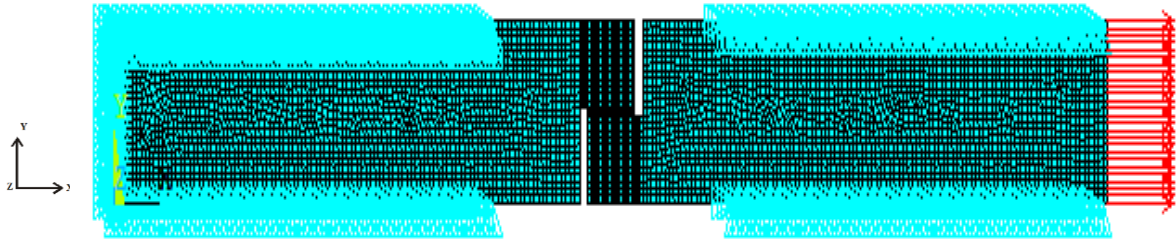
Fig.10.6. Finite element model showing boundary condition
