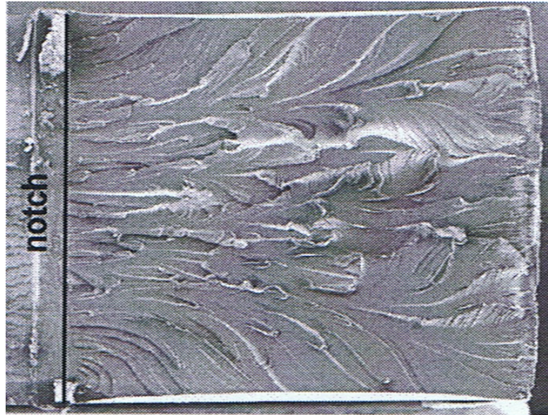
Fig. 5.13 SEM of stretch zones on modified DGEBA resin with low viscosity (Kanchanomalet et al. , 2005).
