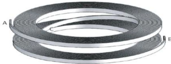
Figure 6-19 Schematic view of a double-pancake coil.
