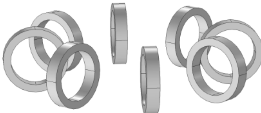
Figure 6-20 Illustration of toroidal SMES configuration.
