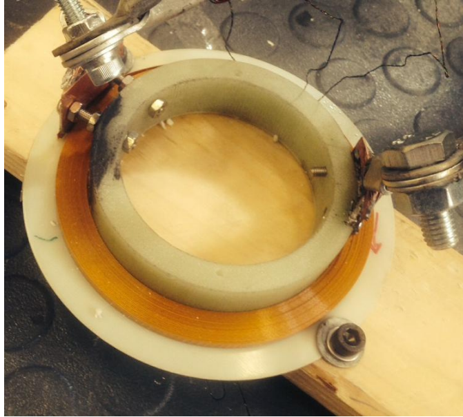
Figure 4-2 The 50-turn coil with SuperPower tape for self field experiments. The inner diameter of the coil is 89 mm and the outer diameter is 110 mm.
