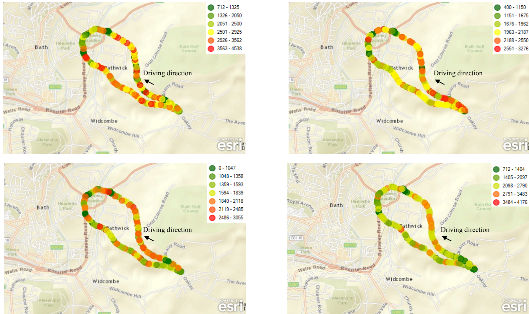
Figure 68. Geo-analysis of the Nissan Note drivers' engine speeds, the maps are based on individual driver's data; the units are in rpm: Driver 9 (top left), Driver 10 (top right), Driver 12 (bottom left), and Driver 13 (bottom right)
