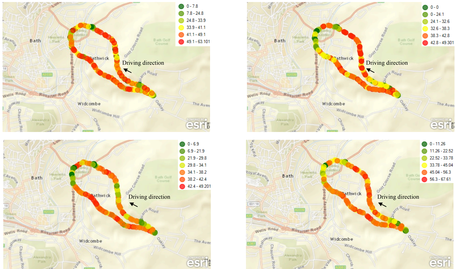
Figure 67. Geo-analysis of the Nissan Note drivers' vehicle speeds, the maps are based on individual driver's data; the units are in km/h: Driver 9 (top left), Driver 10 (top right), Driver 12 (bottom left), and Driver 13 (bottom right)
