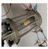
The three taps on the right of the triaxial cell are for two taps on the left are for pressure transducers for the cell pressure and two back pressure lines. The measuring cell and pore pressures
