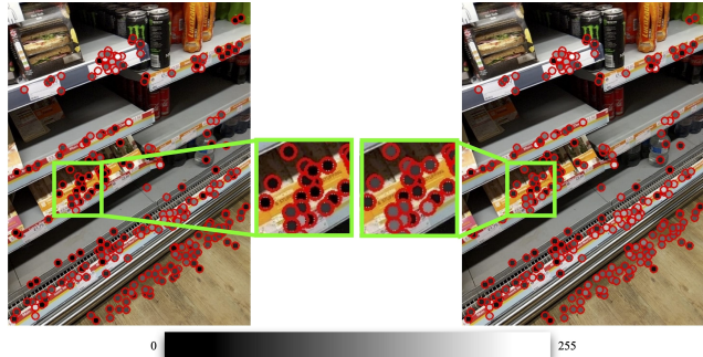
Figure 4. To illustrate the difference between our proposed time-infused score and the plain visibility score (i.e. the number of cameras a point was viewed from), we selected a random picture from the live map and project the map onto it. Each point here is associated with a stability score \sigma^i (left image) and a visibility score v_1 (right image). The higher the value, the more stable the point is. Most of the products’ points from the left cropped-image are darker from the ones in the right. This confirms our hypothesis, that those points on the products (i.e. dynamic objects) are less likely to be used for pose estimation using our score \sigma^i .
