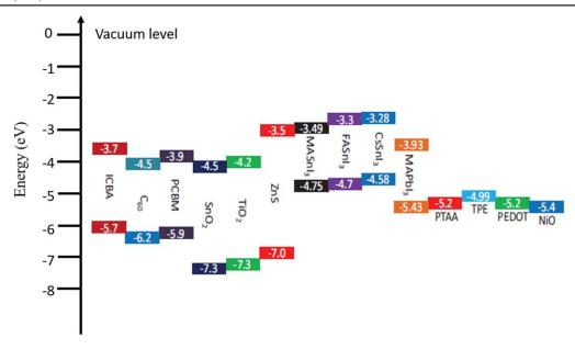
**Figure 20.** Energy diagram of Sn- and Pb-based perovskites along with some common ETLs and HTLs. Unit is in eV. The energy levels are estimated from Tauc plots and photoemission spectroscopy in air. [19] John Wiley & Sons. © 2018 WILEY-VCH Verlag GmbH & Co. KGaA, Weinheim.
