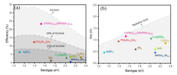
Figure 23. (a) The highest efficiencies and (b) the corresponding  $V_{\rm OC}$  from various PIM-based PV devices reported in the literature to date. The highest values reported in Pb-based perovskite ((FAPbI<sub>3</sub>)<sub>0.95</sub> (MAPbBr<sub>3</sub>)<sub>0.05</sub>) counterpart are also depicted.
