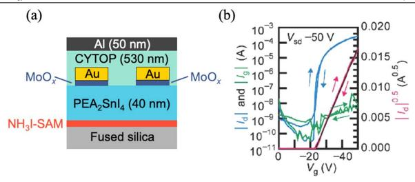
Figure 26. (PEA)<sub>2</sub>SnI<sub>4</sub> perovskite TFTs: (a) device structure and (b) transfer curves. [465] John Wiley & Sons. © 2016 WILEY-VCH Verlag GmbH & Co. KGaA, Weinheim.
