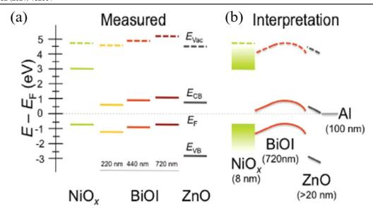
Figure 21. (a) The measured energy alignment of device stack and (b) schematic energy band diagrams for inverted BiOI solar cells. Reproduced from [201]. CC BY 4.0.
