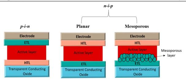
Figure 19. Illustration of the most common device structures used for perovskite-inspired materials.
