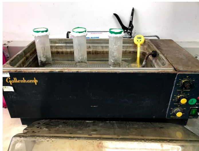
Figure 3-18: Gas permeability experimental set up with cells in the water bath at 40°C
