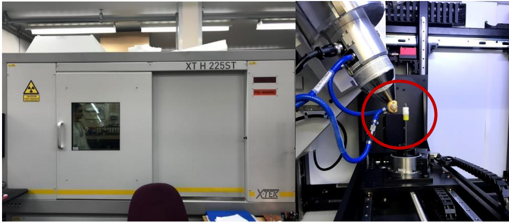
Figure 3-11: \mu CT device (left) and sample positioning under the X-Ray source (right).
