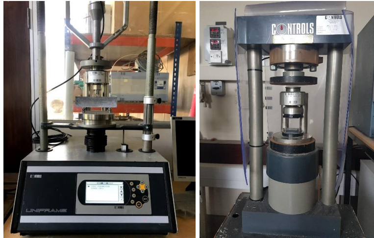
Figure 3-15: Flexural strength (3-point bending) (left) and compressive strength testing (right)
