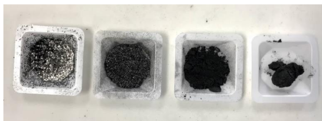
Figure 3-2: Photos of GRMs used in this study (excluding the i-lab materials). From left to right: coarse graphite, medium graphite, fine graphite, graphite nanoplatelets (GNPs)
