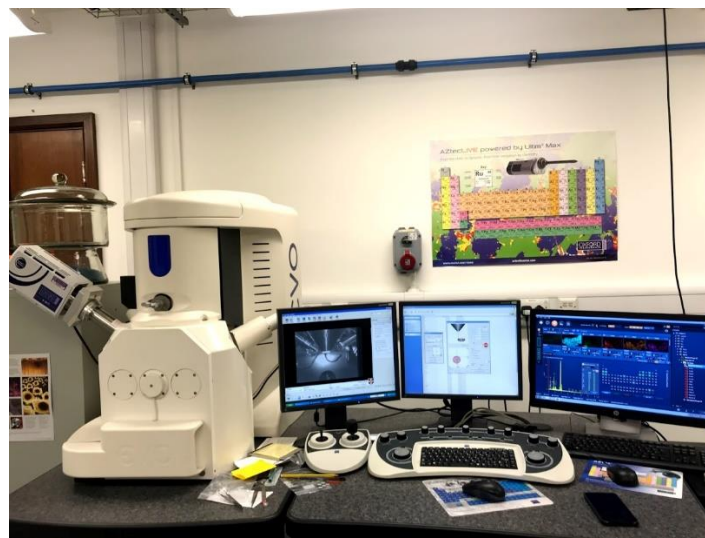
Figure 3-10: ZEISS EVO LS 15 scanning electron microscope (SEM-EDS) used for investigating the dispersion of the GRMs and the microstructure of the composites
