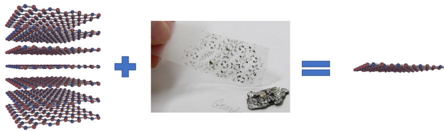
Fig. 2.18 The crystal structure of hBN is identical to graphite, but with carbon atoms replaced by boron (blue spheres) and nitrogen (red spheres). Individual layers can be easily separated via mechanical means such as the scotch tape method due to weak interlayer forces. Adapted Materials World magazine, "Why Boron Nitride Could Be the New Carbon", copyright Institute of Materials, London, UK.
