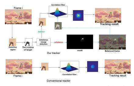
Figure 3: Comparison of our proposed energy-aware CF-based tracker (EACOFT) and the conventional tracker.
