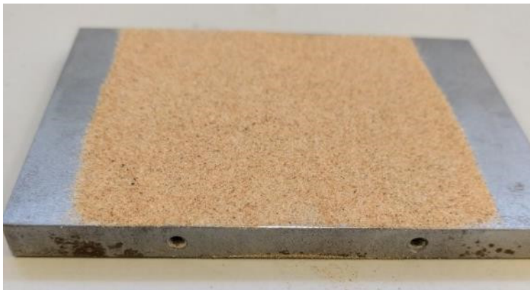
Figure 3-9. Foundation analogue with “single grain thick” sand layer, prior to testing
