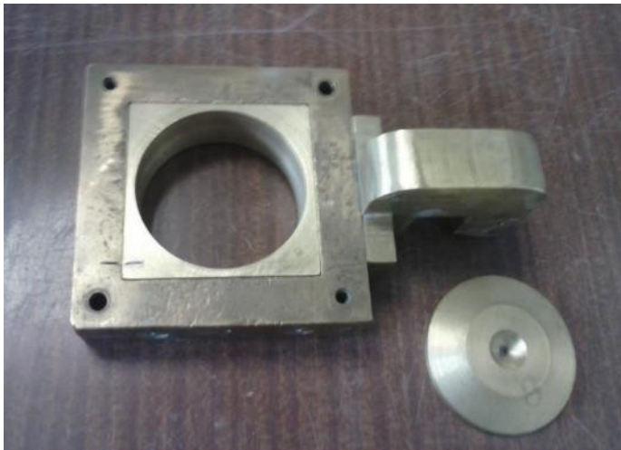
Figure 3-4. Fitting assembly used to accommodate cylindrical samples for shear box testing
