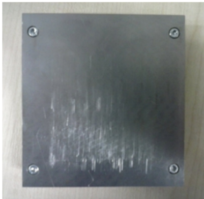
Figure 3-3. Steel block, used instead of bottom half of the shear box
