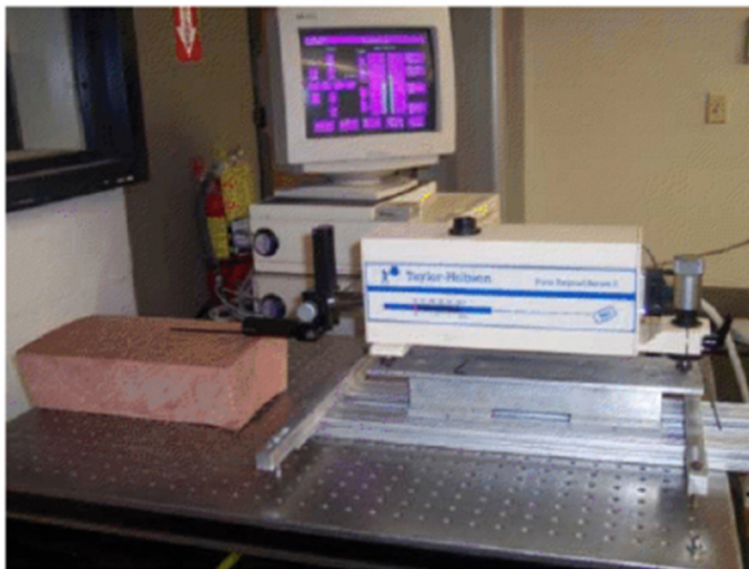
Figure 3-27. Taylor-Hobson Talysurf series 2 stylus profilometer (Source: Iscimen and Frost 2008)
