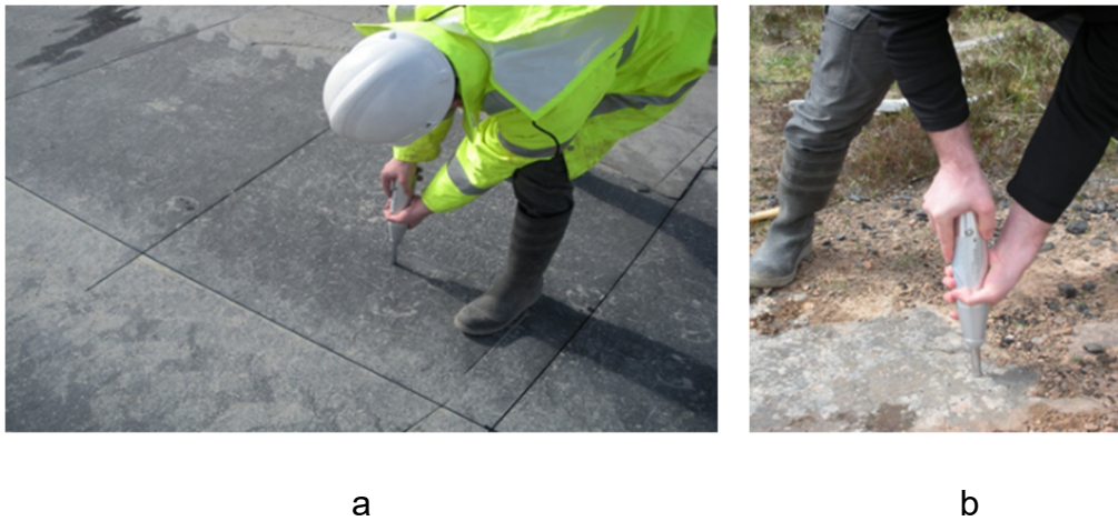
Figure 3-19. In-situ recording of the rebound hardness number (N) using an L-type Schmidt Hammer. (a) Caithness Flagstone (ND07829 63333), (b) John O'Groats Sandstone (ND37150 70138)
