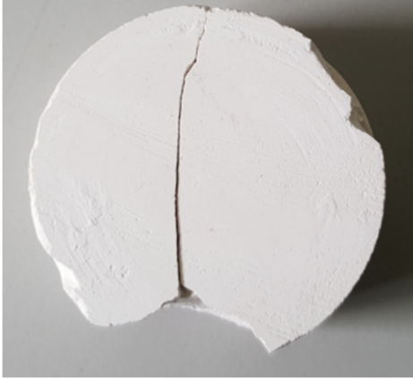
Figure 7-8. Tensile failure of a dry Chalk sample sheared at 1000 kPa
