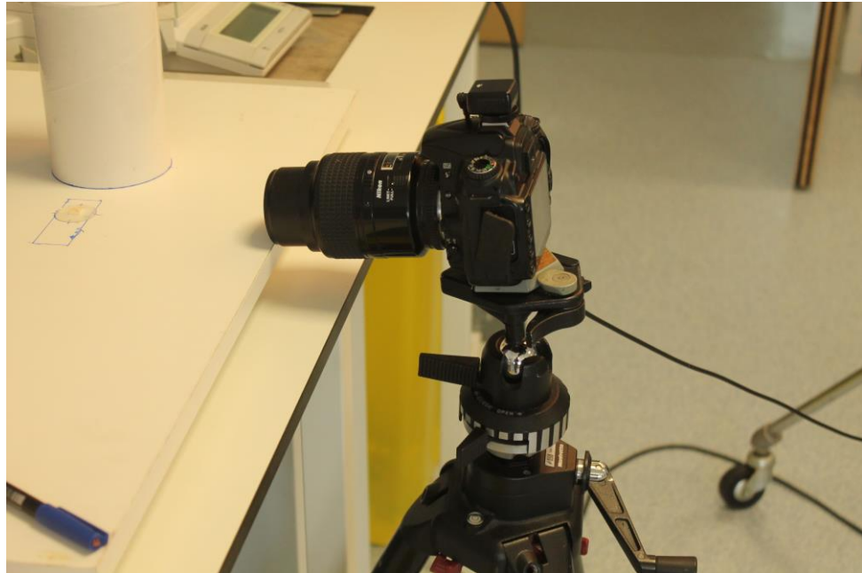
Figure 3.5. Camera set up to capture image of static contact angle
