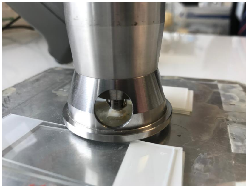
Figure 3.11. Vickers diamond contacting sample
