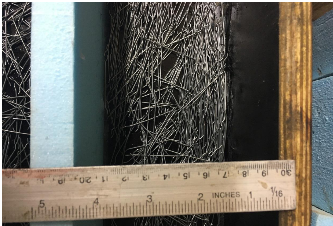
Figure 3.22 Alignment of the steel fibres as a layer in the casting mould
