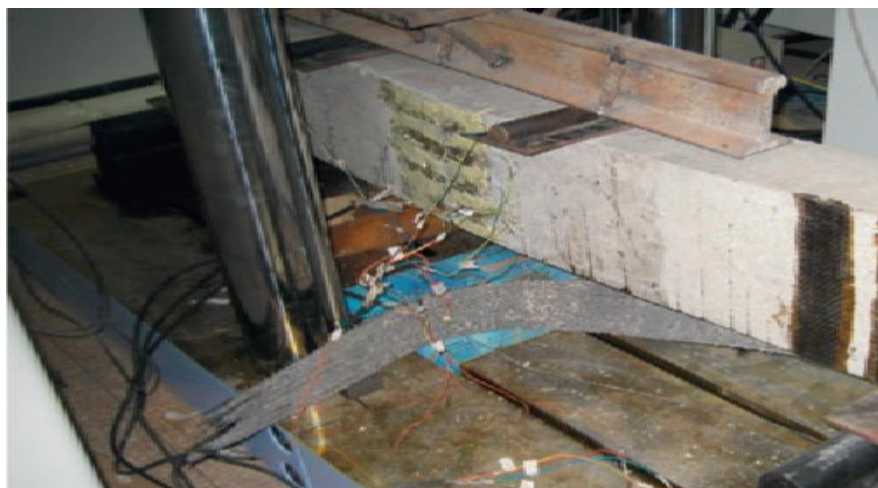
Figure 2.7 Failure of beam strengthened with external CFRP sheets (Dong, et al., 2013)
