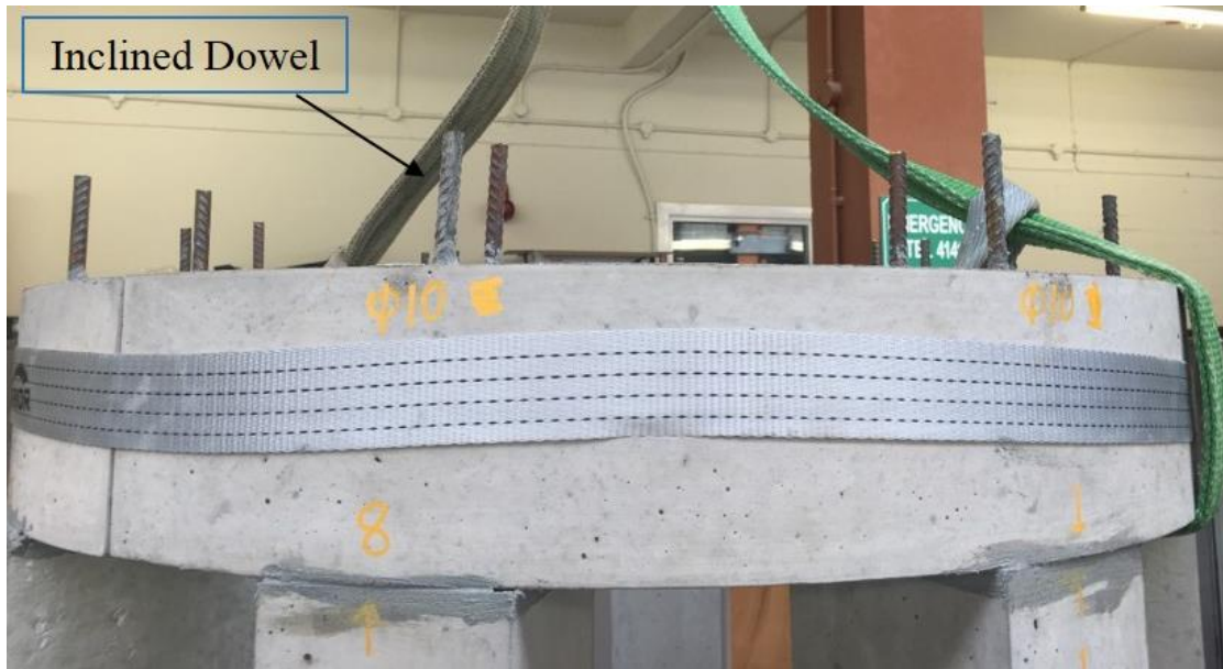
Figure 7.9 The middle dowel connectors staying out for final jointing
