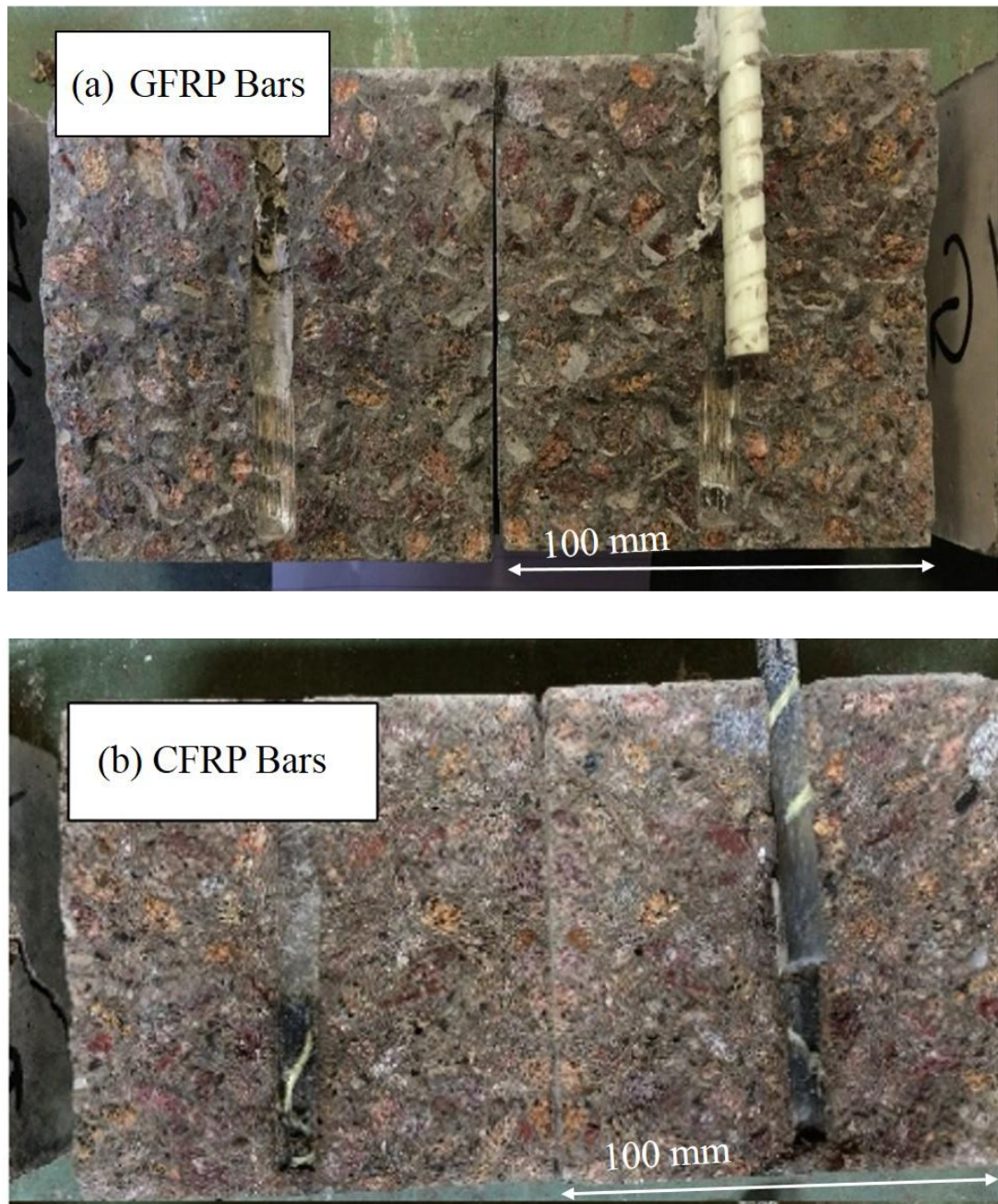
Figure 4.2 Failure of the pull-out test specimens after splitting the concrete cubes: (a) GFRP bars and (b) CFRP bars
