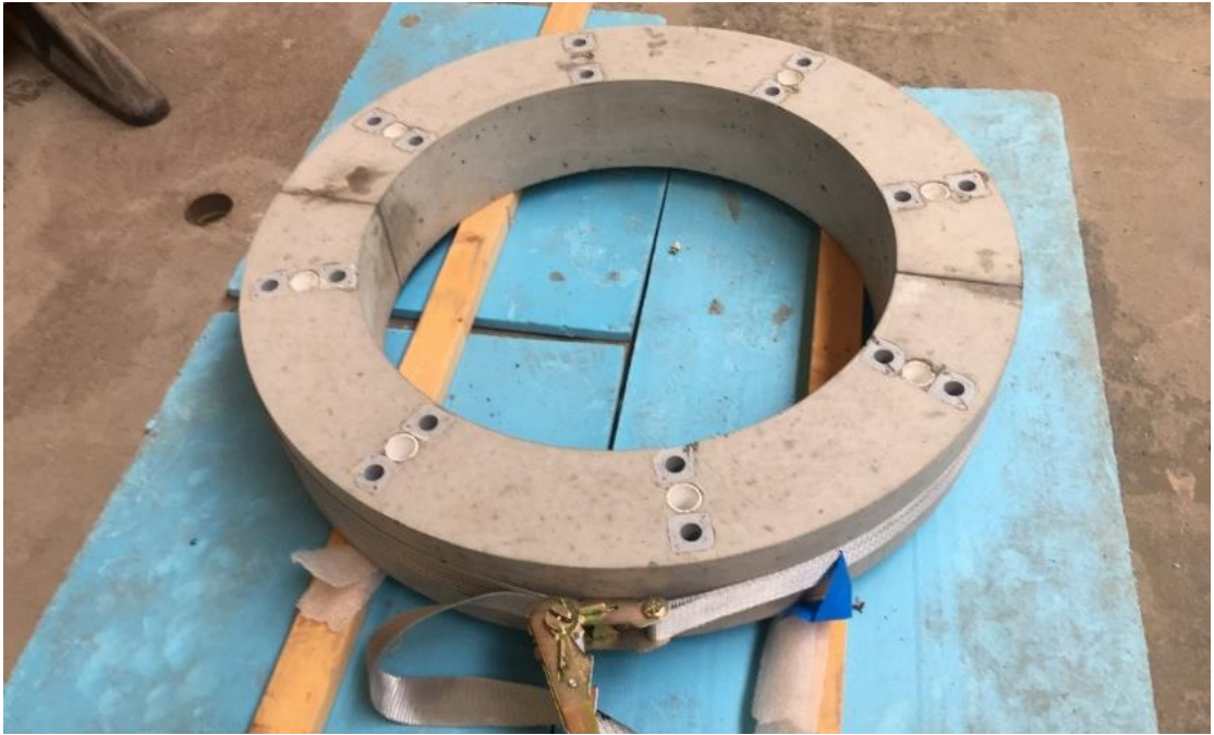
Figure 7.7 Joining of the ring section with the ratchet strap
