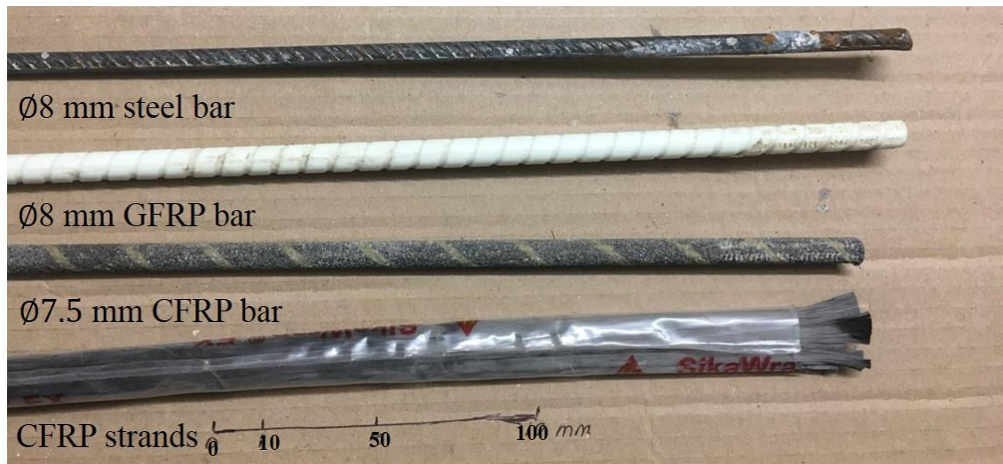
Figure 3.2 GFRP bar, CFRP bar and CFRP strands compared with an 8 mm steel bar
