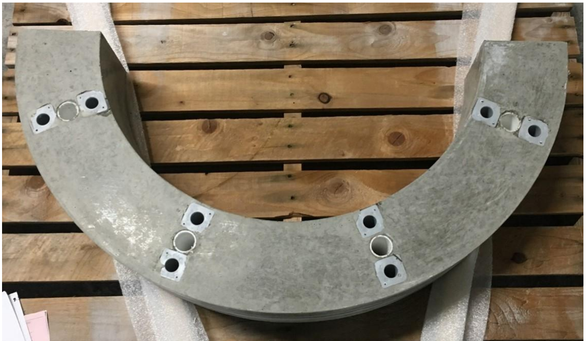
Figure 3.34 One half ring component after demoulding in Plean Precast Ltd.
