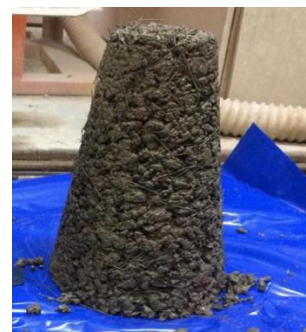
Figure A.3 The fresh mixed concrete of Trial I in the pan before the slump test (left), and slump test for the mix of Trial II (right)
