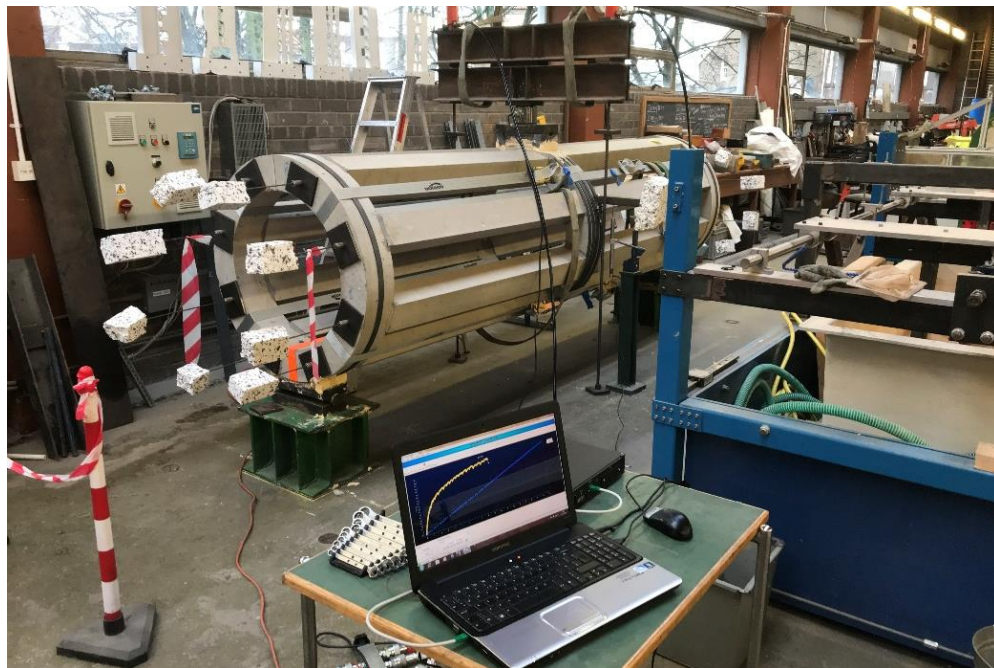
Figure 7.15 Three-point bending test on the assembled and steel-wire post-tensioned (1 MPa) truss (taken by Dr. L. Zheng)
