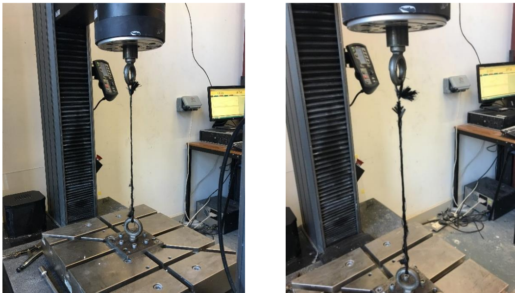
Figure 4.11 Test setup (left) and failure (right) of the CFRP strands under the tensile test
