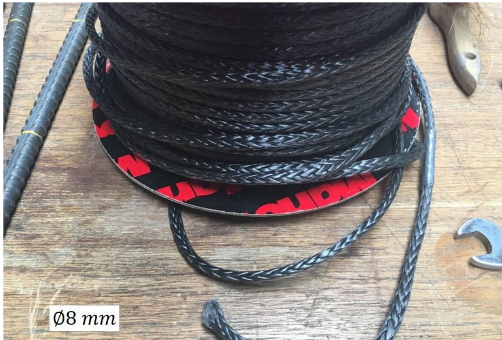
Figure 7.1 The Marlow ® D12 SK99 product as the reinforcing ropes for the prototype
