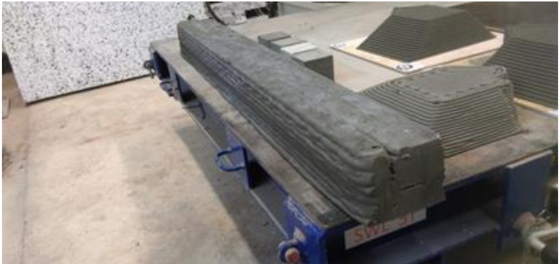
Figure 3.36 The 3D printed beam arrived at the University of Dundee laboratories
