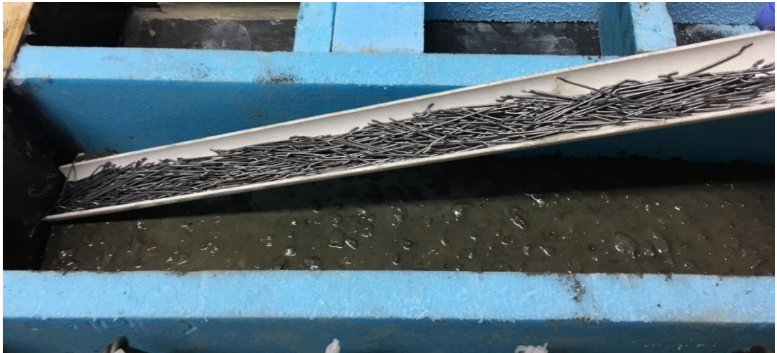
Figure 3.9 Transferring the aligned steel fibres from the PVC gutter to the mould
