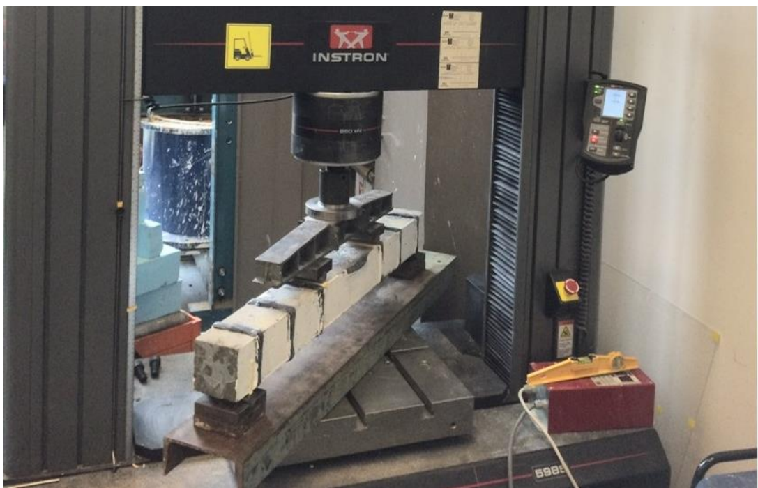
Figure 3.20 Test setup of the jointed CFRP beam specimen
