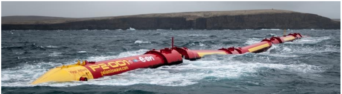
Figure 2.1 The cylindrical-tube-type Pelamis WEC prototype P2-001 floating on the sea (European Marine Energy Centre, 2017)
