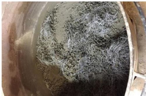
Figure A.3 The fresh mixed concrete of Trial I in the pan before the slump test (left), and slump test for the mix of Trial II (right)
