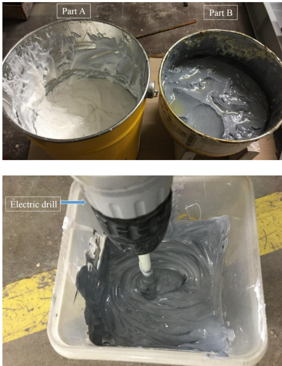
Figure 3.4 Epoxy resin adhesive before (above) and during (below) the mixing
