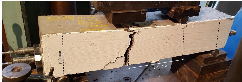
Figure C.3 Crack and failure of one post-tensioned beam reinforced with GFRP
