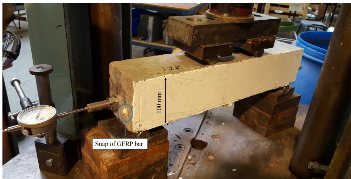
Figure 3.25 Snap of the GFRP bar after post-tensioning
