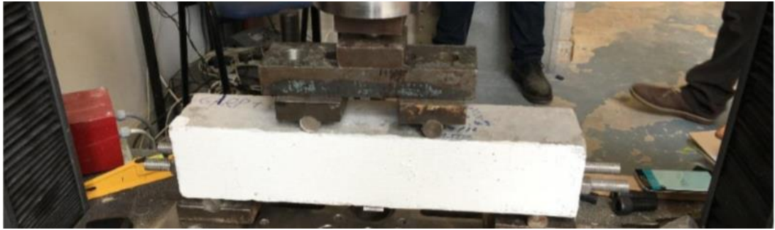
Figure 3.17 Test setup of the four-point bending test with the Instron machine
