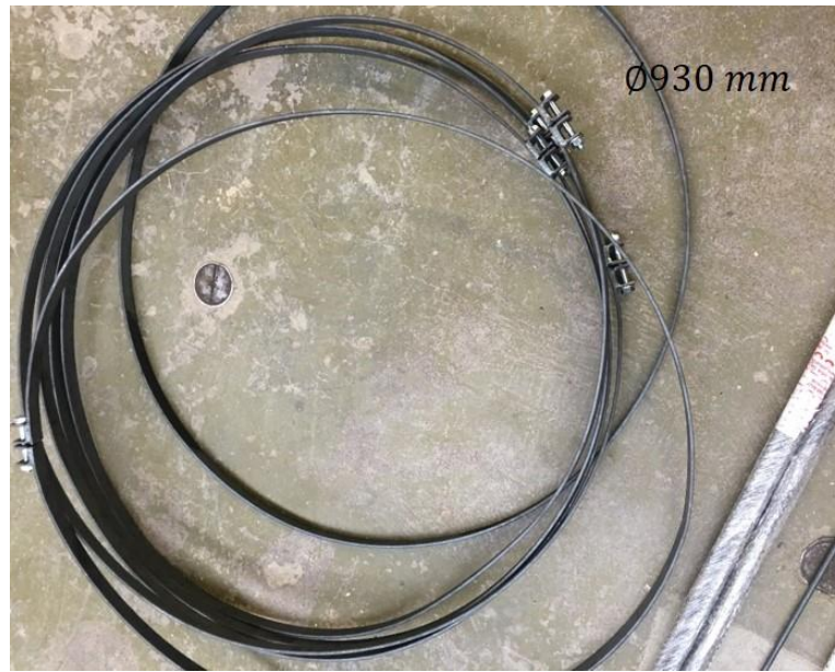
Figure 7.11 The manufactured steel band confinement with an adjustable and securing M12 screw
