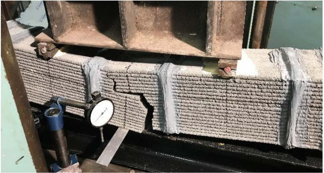
Figure 7.5 Crack of the 3D printed beam under the bending at a deflection of 6 mm (taken by Dr. L. Zheng)
